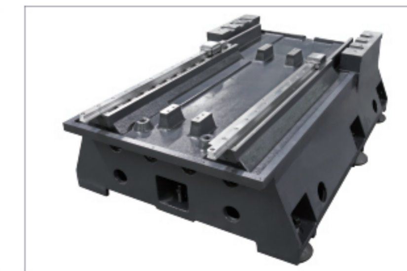
Double layered box type base
