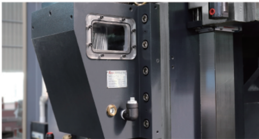
Two-speed gear head (spindle can be equipped with a two-speed gear head)
