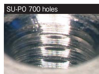
Roughness of thread flank face Ra=2.0 μm
