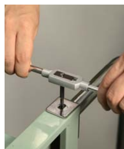
When hand tapping, always use tap wrench
