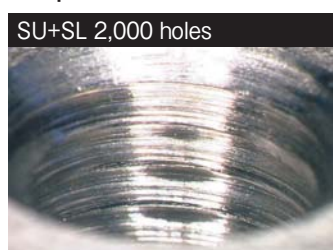
Roughness of thread flank face Ra=1.1 μm
