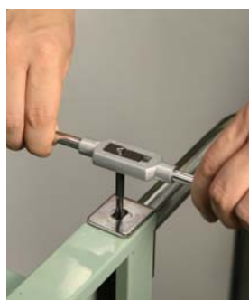
When hand tapping, always use tap wrench
