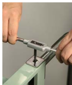
When hand tapping, always use tap wrench
