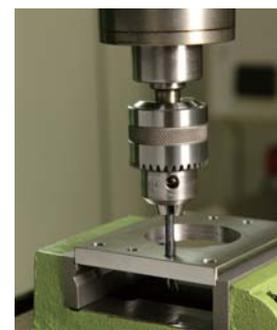
Machine tapping with drilling machine
